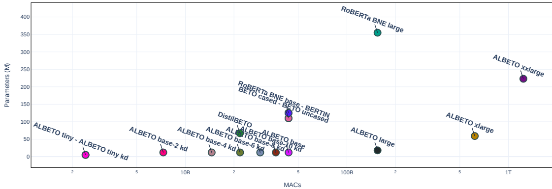
Figure 1: The size (number of parameters) and speed (MACs) of every Spanish model evaluated on this work. MACs are measured using a single sequence of length 512, which is the maximum sequence length of all the evaluated models.
